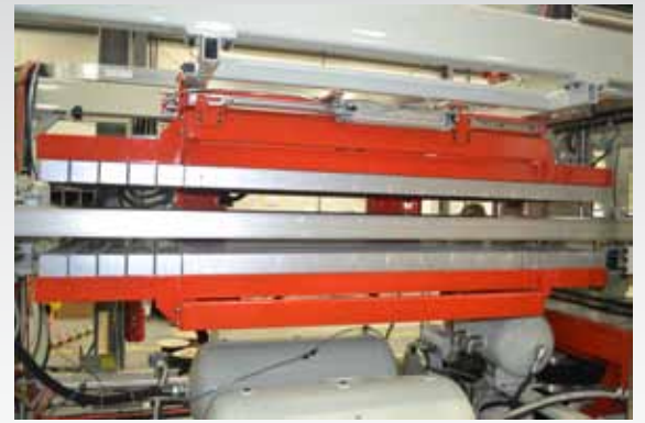
Oven is four times the index length of the forming area and incorporates high efficiency heaters
