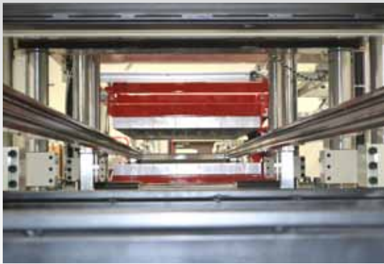
Extra length between forming and cutting stations to allow sufficient cooling when processing PP
